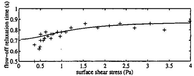
Figure 10. Comparison of measured flow-off relaxation time (symbols) and theoretical prediction (solid line).
