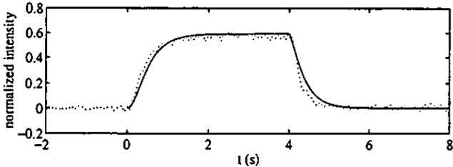
Figure 8. Comparison of measured intensity history (broken line) and theoretical prediction (solid line).
