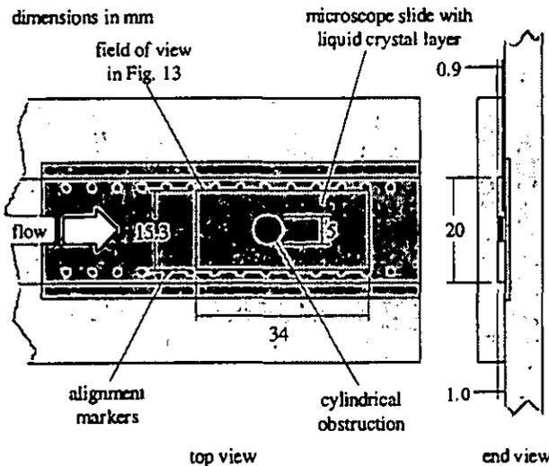
**Figure 12. Laminar flow duct configuration for the cylindrical obstruction experiments.**
