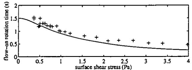
Figure 11. Comparison of measured flow-on rotation time (symbols) and theoretical prediction (solid line).
