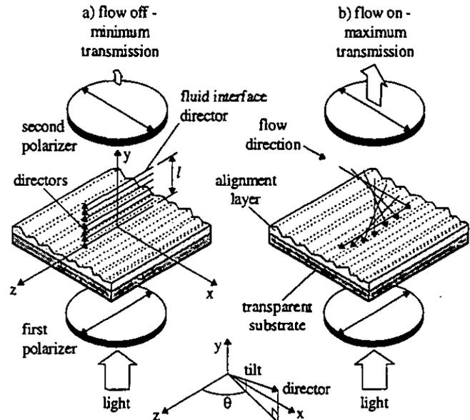
Figure 1. Illustration of the liquid crystal technique.
