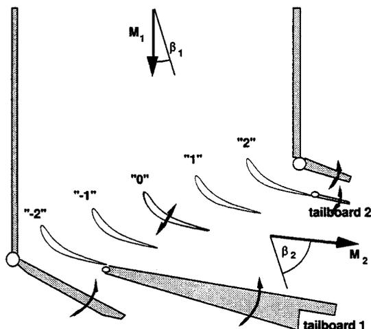
Fig. 1: Schematic view of the linear test facility
